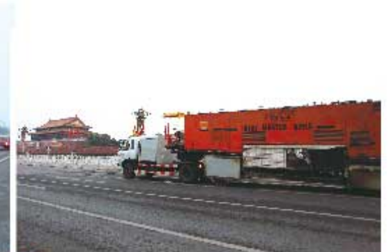
Daily pavement recycling capacity upto 16,000 m 2 .
