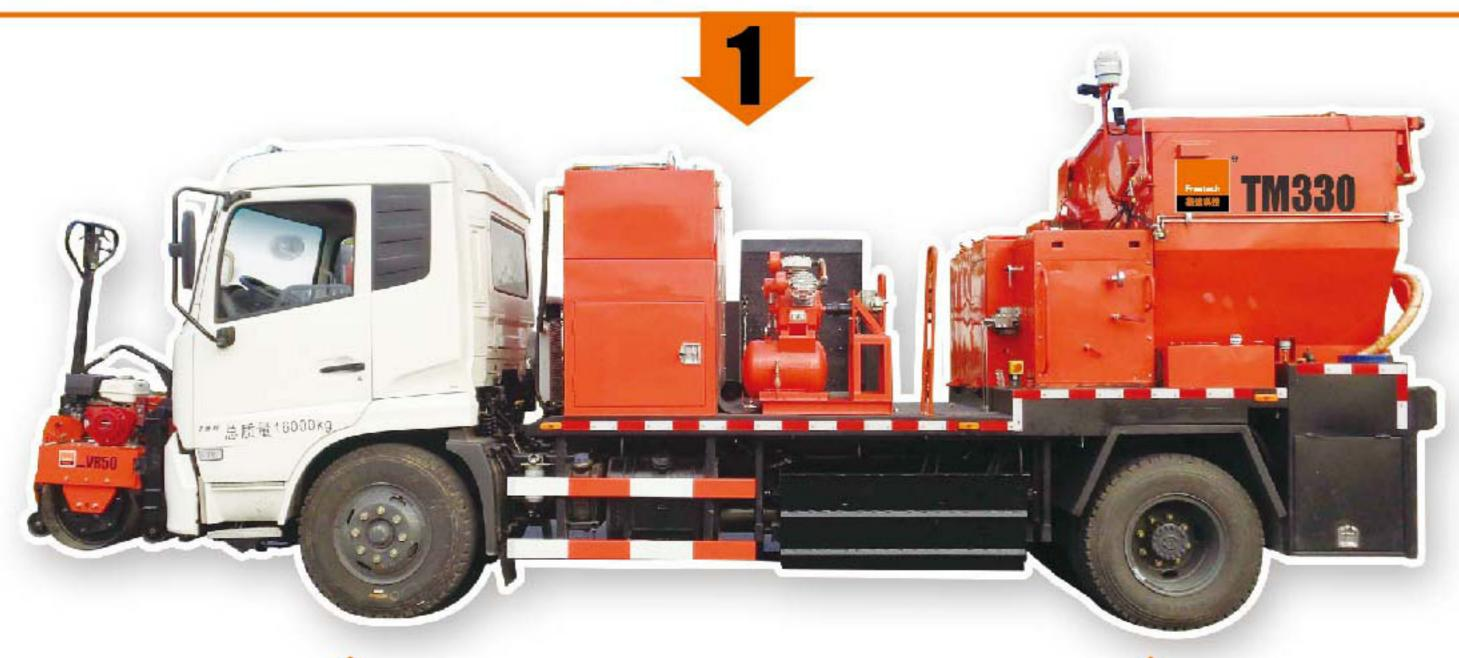
Large capacity sealant melter applicator for crack sealing
